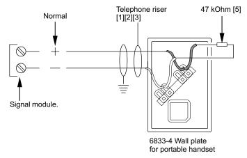
[4] Connect the shields to chassis ground in the control panel
