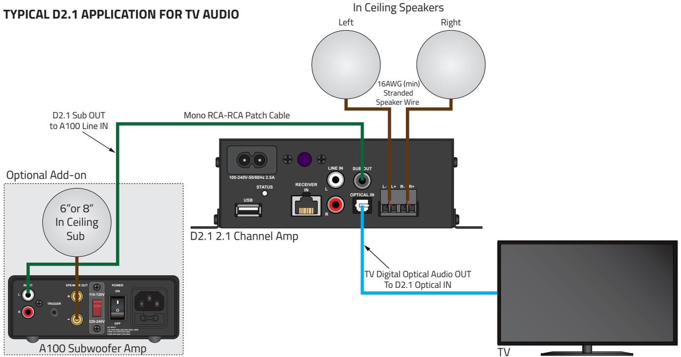
Typical System application for stereo audio and subwoofer. Amp will auto-sense TV audio (or other source) and output audio to speakers and sub amp automatically. Amp can be hidden in a cabinet and controlled via IR Repeater system using either the D2.1 IR Remote or TV Remote.
