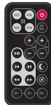
The D2.1 IR Remote is a full-featured, 'credit card' remote. It includes all D2.1 functions including power, input, master volume, sub volume, mute, four EQ settings and night mode. It also features IR commands that can control a compatible Bluetooth device that is synced to the Bluetooth Module.
