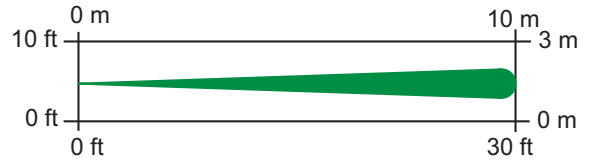
Side View Optional Pet Coverage (OLP91): 10 m x 12 m (30 ft x 38 ft)
