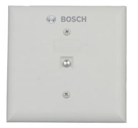
The module connects a normally-open (NO) contact to the multiplex bus of FPD-7024, D7024, or DS9400 Addressable FACPs. Use the D7044 supervised input in a Class B configuration. All operating power for the input module is drawn from the fire alarm control panel (FACP).
