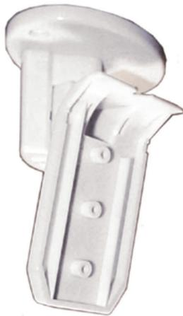
Surface mounts detectors to the ceiling. The vertical pivot range is +7° to -16°; the horizontal pivot range is ±45°. Do not use for pet applications.
