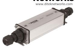
**DITEK's DTK-EXTO** Extends the range of a PoE connection — even in harsh outdoor conditions. The DITEK Networks' Outdoor Gigabit High-Power PoE+ Extender Repeater is designed to extend connection distances from a PoE source to an output device up to 100 m (328 ft.) via Cat5e or Cat6 cable. Cover even longer distances by cascading up to five extenders. The PoE+ Extender Repeater does not need an additional power supply, as it draws the power it needs from the PoE input.
