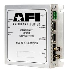
The American Fibertek 46-PoE+ Series transmits and receives (2) copper 10/100/1000BASE-T Ethernet signals at the RJ45 ports and (1) optical 100 Base-FX over 1 or 2 multimode fibers. The system is comprised of two units forming a point-to-point communications link.
