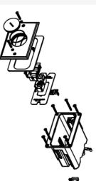
Wiremold WMFB1KS2N Series Single-Gang Floor Box Assembly Part No. WMFB1KS2N
