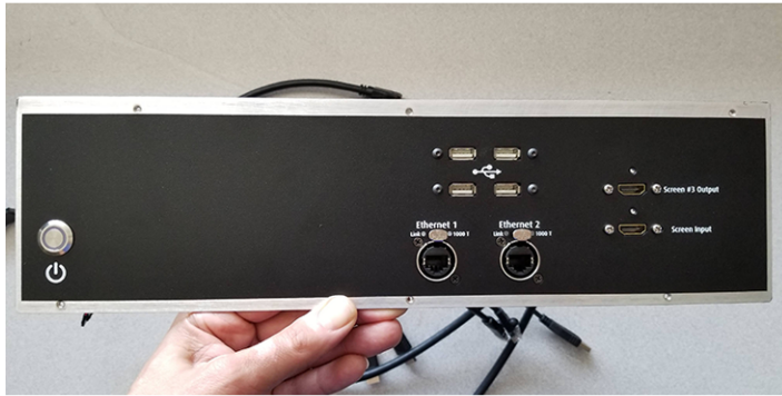
Image 2-13: EC-210 rear I/O plate with connections
