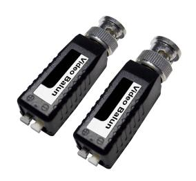
Single-channel passive video balun enables full motion video transmission over UTP up to 2,000', or 3,000' if used with an active receiver. Compatible with analog or HD. Easy installation with push terminals and BNC connector. One pair per package.
