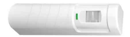
Model OE-RXDST is an advanced Request-to-Exit (REX) motion detector that provides door control via a door control device (such as magnetic lock or door strike) or access control system. A variety of programable options allows customization to suit the application. Sequential triggering allows for a higher degree of security and a door alert sounder is included. Durable ABS plastic housing. Optional trim plate (OE-TP) facilitates neat installation, especially with single gang box.
