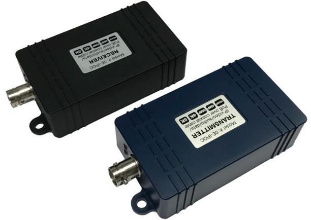
IP over Coax transmitter and receiver set enables use of existing coax cable to upgrade to transmission of IP video, audio and data with PoE. Plug-and-play installation without configuration and compatibility with IEEE802.3af and IEEE802.3at PoE protocols simplify upgrades from analog to IP.
